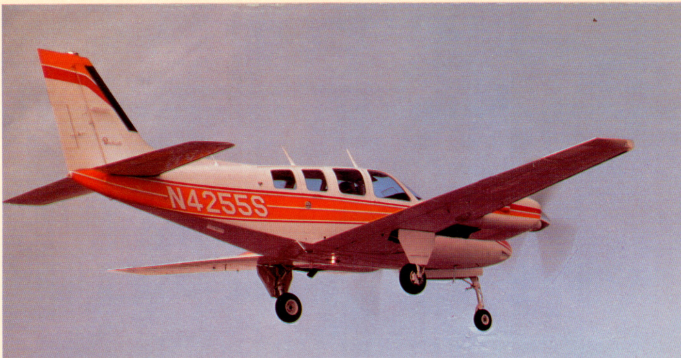
Gear down speed of the B58 TC is 177 knots. Access to the rear cabin is through a double door at the trailing edge of the wing.
